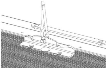
Tighten the staples/spikes puller with one hand by pulling the handle upwards.
